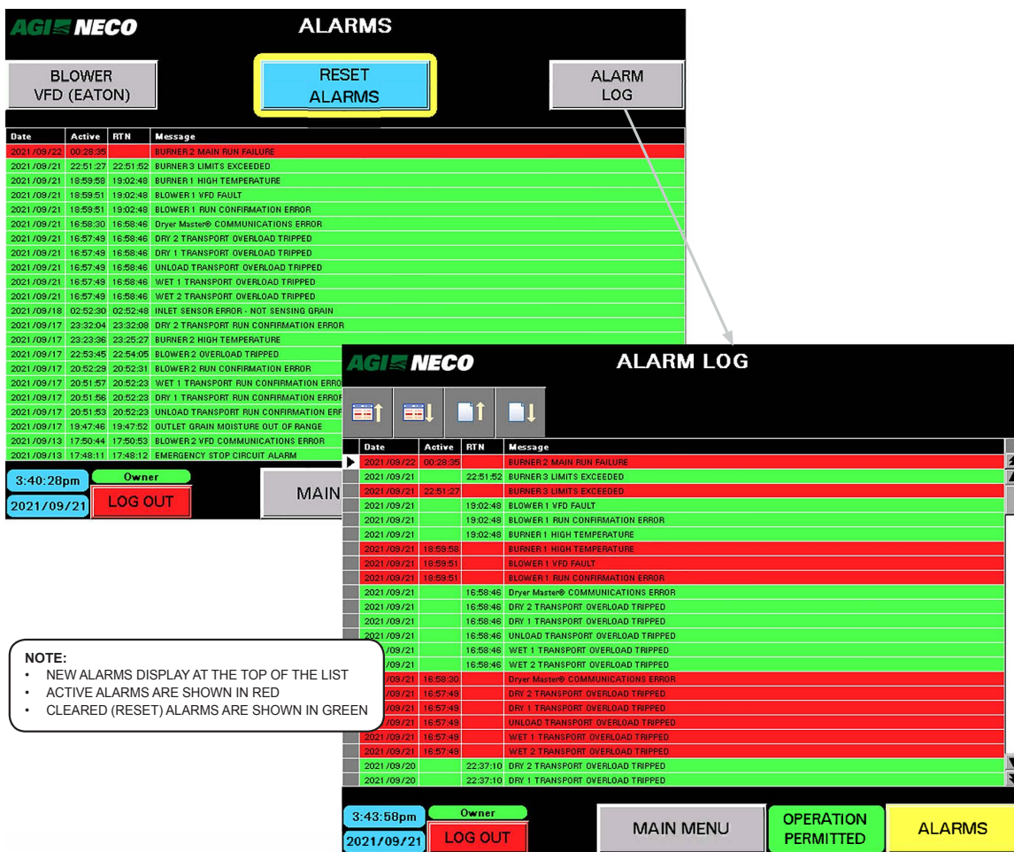
Figure 95. Alarms and Alarm Log Screens
